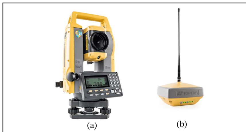
Figure 1. (a) Total station, (b) GNSS instrument in data collection
