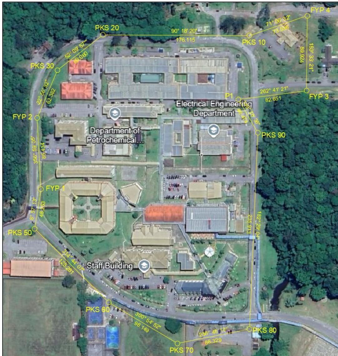
Figure 5. Overview of the 13 traverse observation stations including the New Datum.
