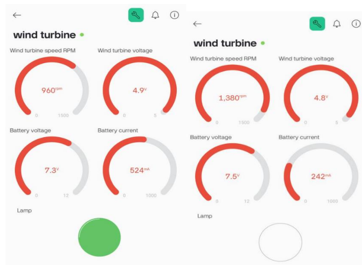
Figure 3 : Measurement display using Blynk apps
