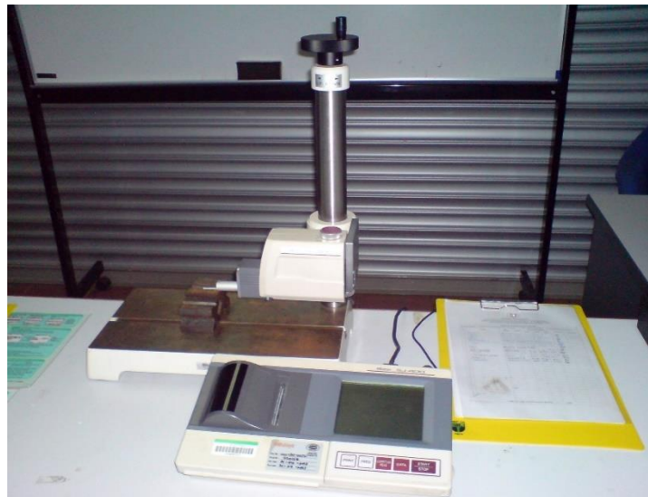
Figure 3. Mitutoyo Surface Roughness Measuring Set
