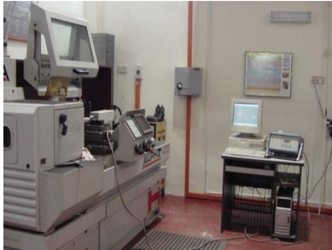
Figure 2. Numerical Control Lathe fitted with Kistler force dynamometer.
