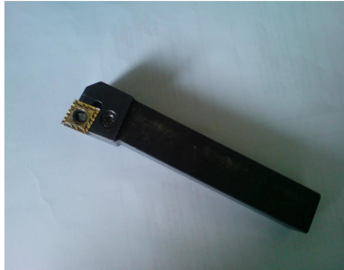
Figure 1. Solid Coated Cemented Carbide Cutting Tool
