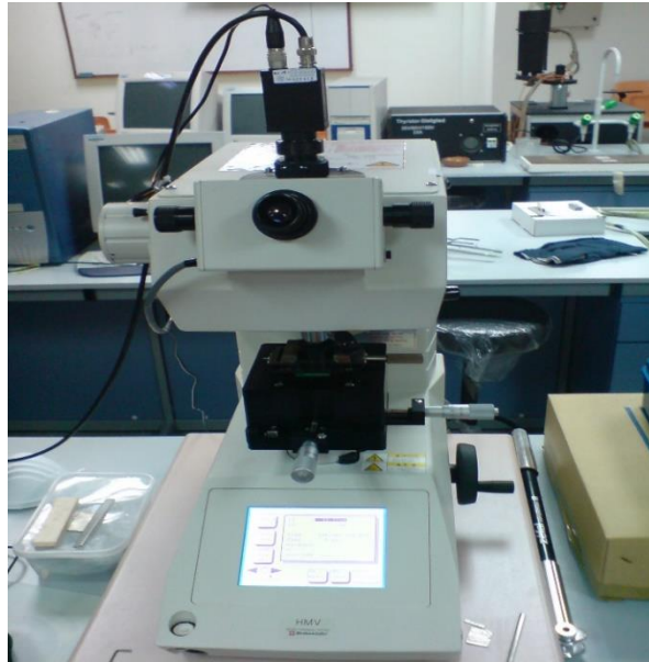
Figure 4. HMV Vickers Hardness Equipment
