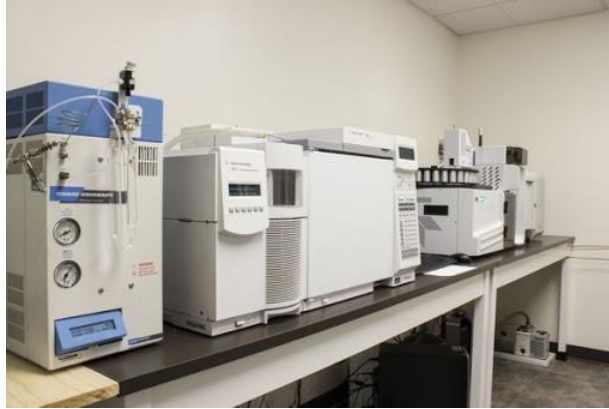
Figure 3: Gas Chromatography - Flame Ionization Detection (GC- FID)
