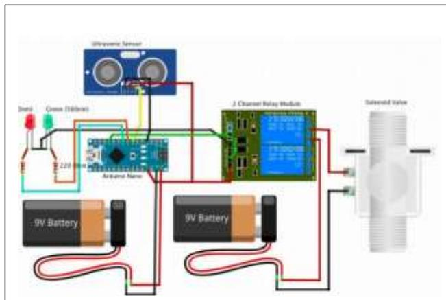
Figure 1. The SMUF's Schematic Diagram
