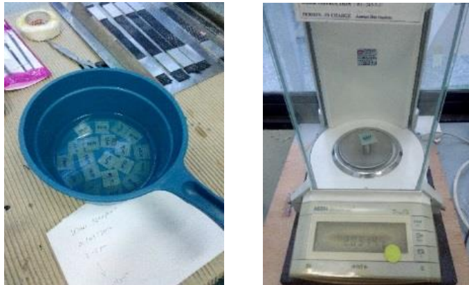
Figure 12. Water Absorption Test
