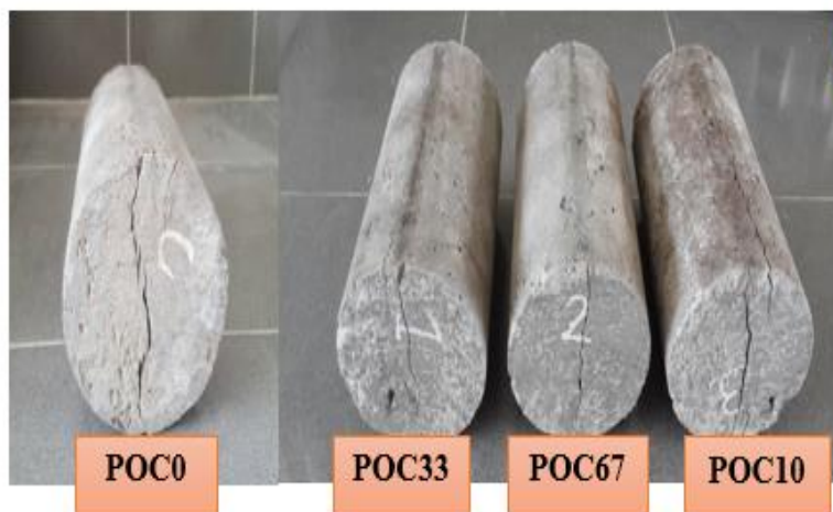
Figure 8. Typical failure pattern of control and POC replacement concrete cylindrical
