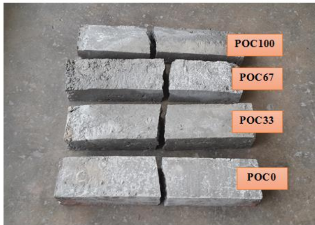
Figure 10. Typical failure pattern of control and POC replacement concrete prism
