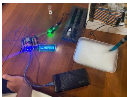
Figure 5: pH sensor testing process
