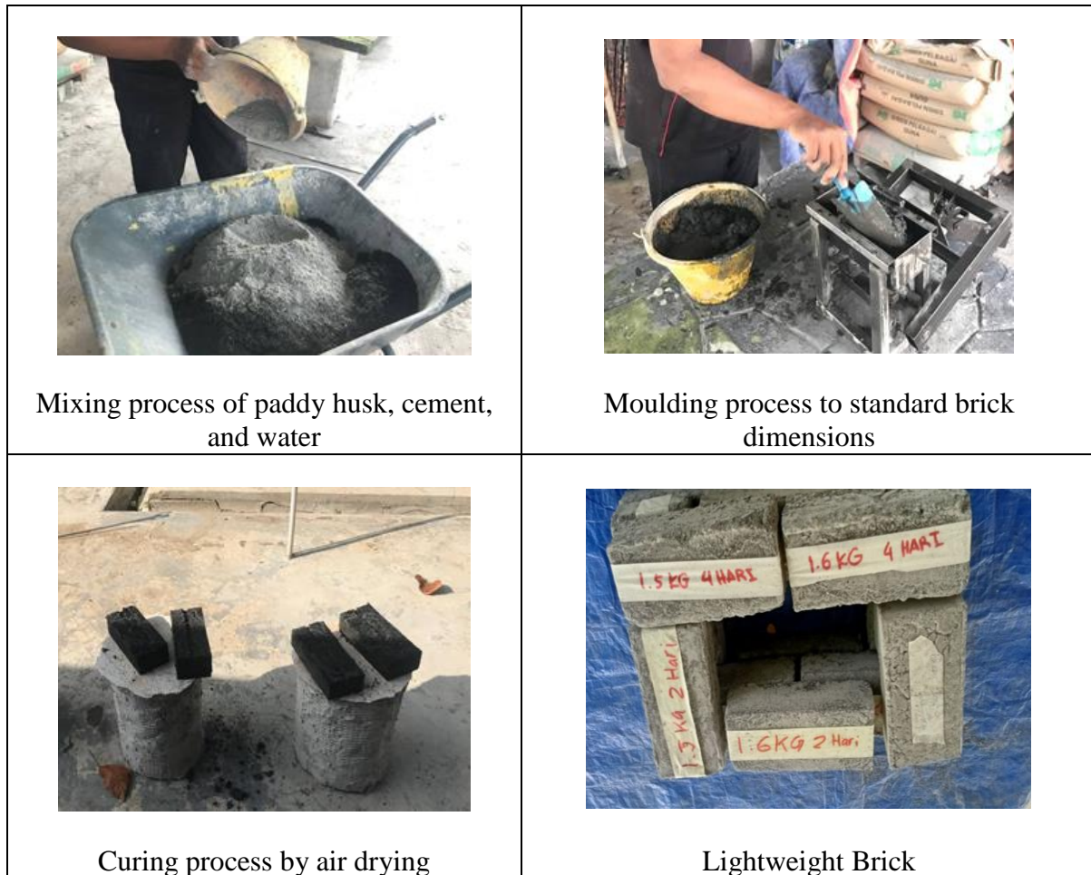
Figure 2. Production process of lightweight brick using paddy husk
